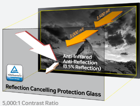
Figure 1. High brightness and contrast ratio suited for outdoor environment
